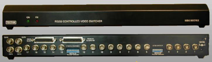
This is a small matrix controlled by RS232 commands. Any one of the 17 inputs can be connected to any of the four outputs. When linked with a Darlex multiway keyboard, 17 up to 34 Darlex Digital Recorders can be controlled and viewed from one position. Multiple RS232 controlled switchers can be linked together. The Switchers are controlled from our keyboards or your own electronics/PC.
